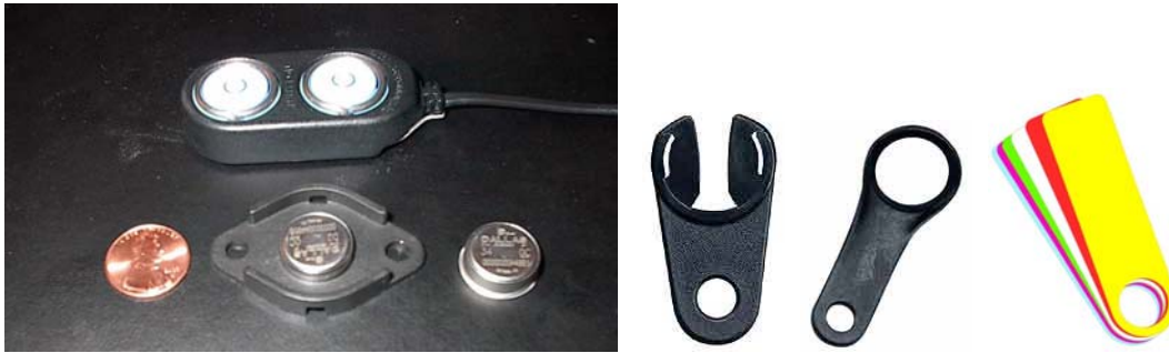
Figure 2 – Photo of the Q-Efficient™ Hold-In-Place Reader and Fobs for attaching the iButtons to Gauges
